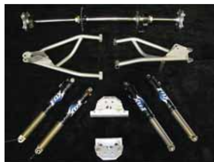
Image is of Front and Rear Suspension: need to Order DFR-2170RLT for Rear Suspension. Rear suspension is new Rear Axle, Fox Floats, and new Chain links.
